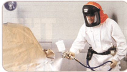
This painter is dressed for both safety and productivity. The overspray stays off the covered painter, and the dirt on the painter stays out of the job. Photo courtesy of SATA USA.
